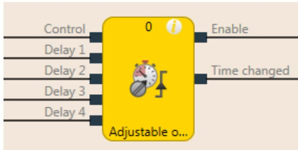
Illustration 88: Function block diagram for the adjustable switch-on delay function block
