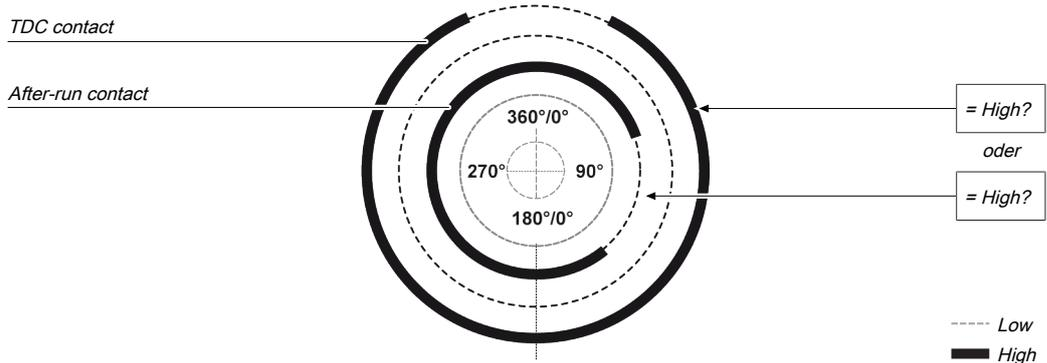
Illustration 139: Contact monitoring with the universal press contact monitor function block with activated ramp-down
