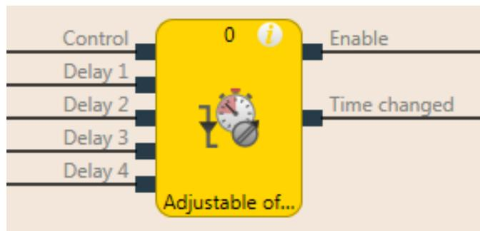
Illustration 84: Function block diagram for the adjustable switch-off delay function block
