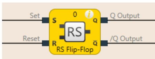
Illustration 53: Logical connections for the RS flip-flop function block
