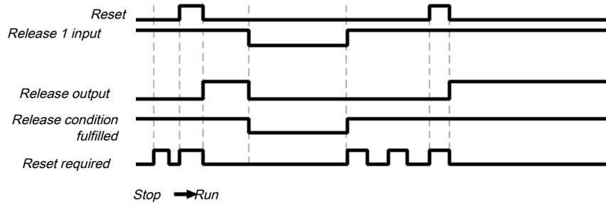
Illustration 213: Flow/Timing diagram for the function block
