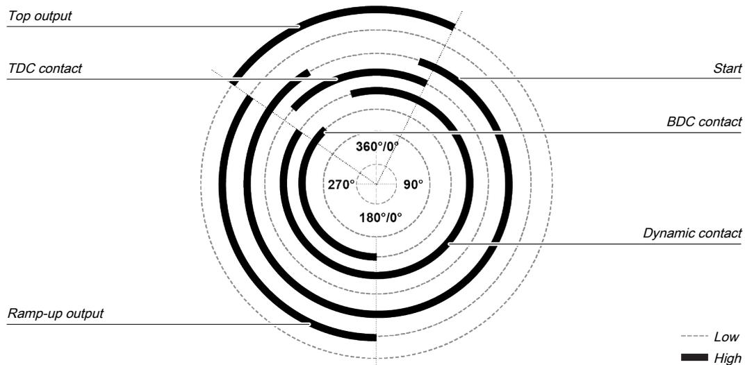
Illustration 146: Contact and output sequence of a universal press during an error-free sequence (example)
