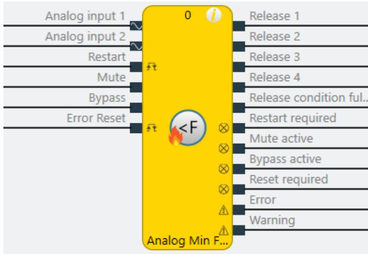
Illustration 187: Logical connections for the Analog min flow function block
