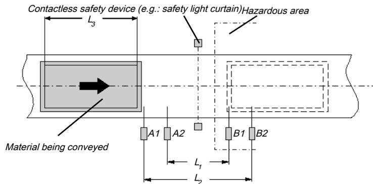
Illustration 124: Example of the sequential arrangement of muting sensors
