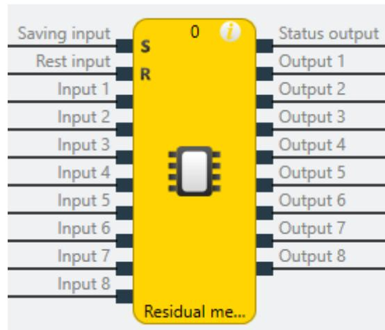
Illustration 77: Function block diagram for the retentive memory function block
