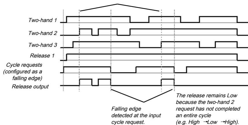
Illustration 116: Sequence/timing diagram for the multi-two-hand function block
