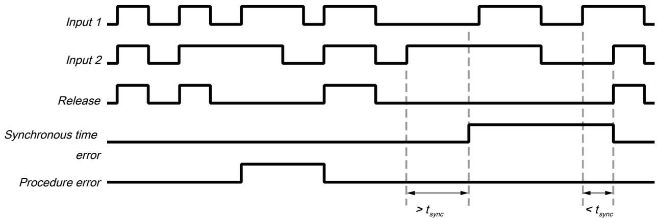
Illustration 106: Sequence/timing diagram for the emergency stop function block
