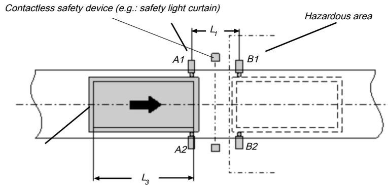
Illustration 121: Muting with two parallel sensor pairs
