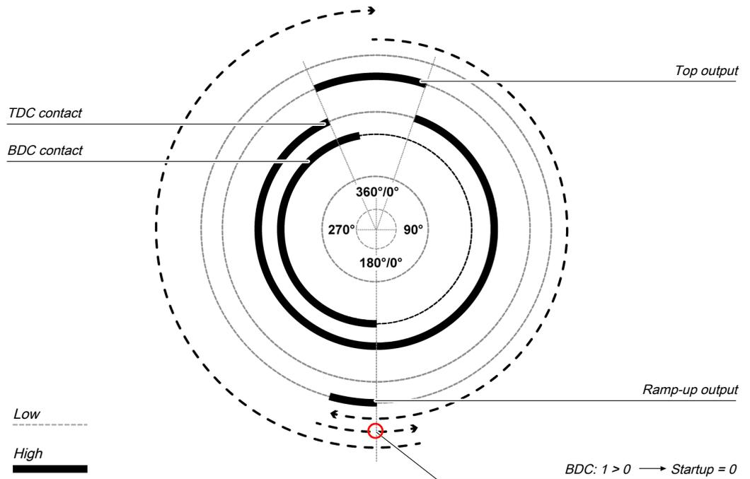
Illustration 143: Press cycle for the universal press contact monitor function block with 2 BDC transitions
