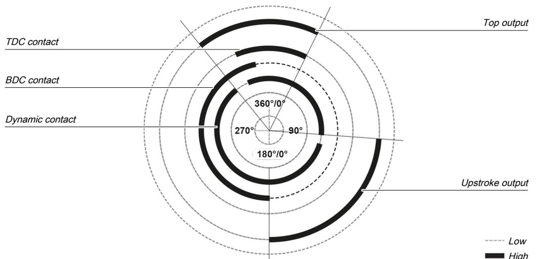
*Illustration 136: Press cycle for the eccentric press contact monitor function block with dynamic contact at startup and for the downward movement*
