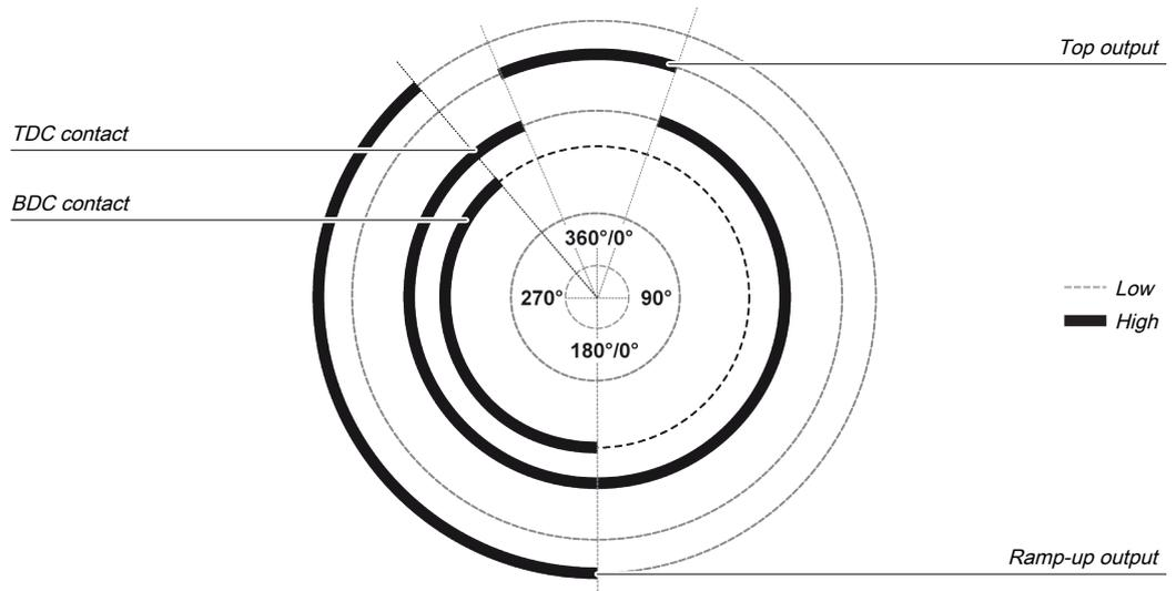
Illustration 142: Press cycle for the universal press contact monitor function block with falling edge of BDC contact before TDC contact
