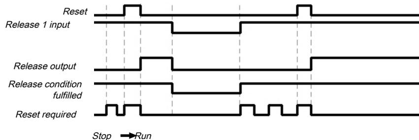
Illustration 217: Flow/Timing diagram for the function block
