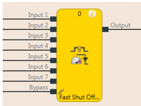
Illustration 60: Logical connections for the fast shut-off with bypass function block
