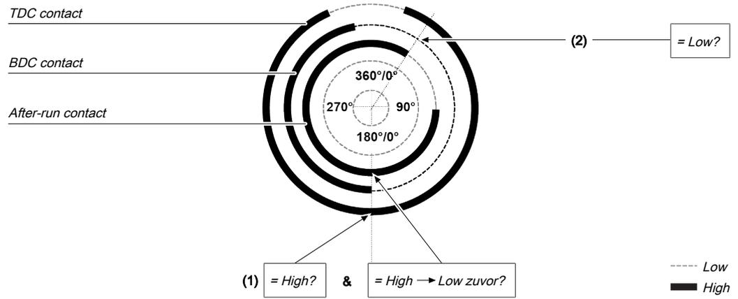
Illustration 145: Contact monitoring with the universal press contact monitor function block with activated BDC contact and ramp-down
