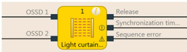
Illustration 108: Function block diagram for the light grid evaluation function block
