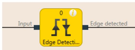
Illustration 67: Logical connections for the edge detection function block
