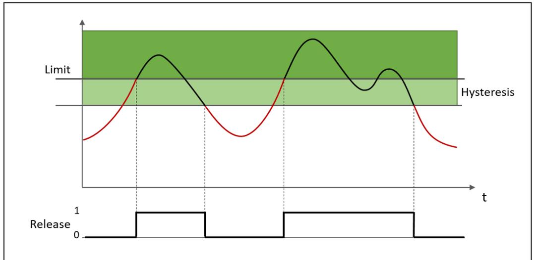
Illustration 195: Monitoring for "Lower limit exceeded"
