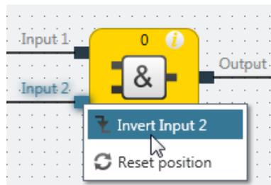
**Display of inverted inputs or outputs**
