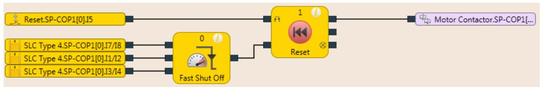
Illustration 61: Configuration example for a fast shut-off with three light barriers
