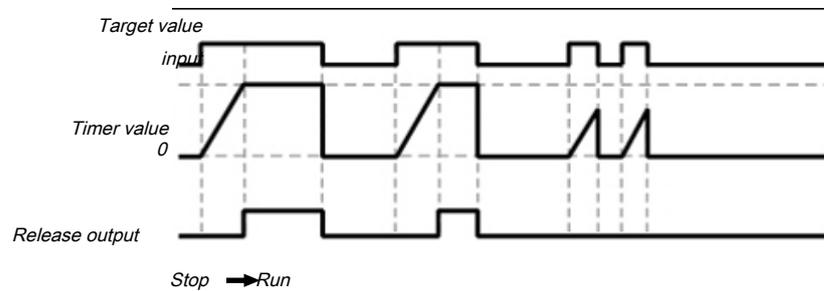
Illustration 87: Sequence/timing diagram for the switch-on delay function block
