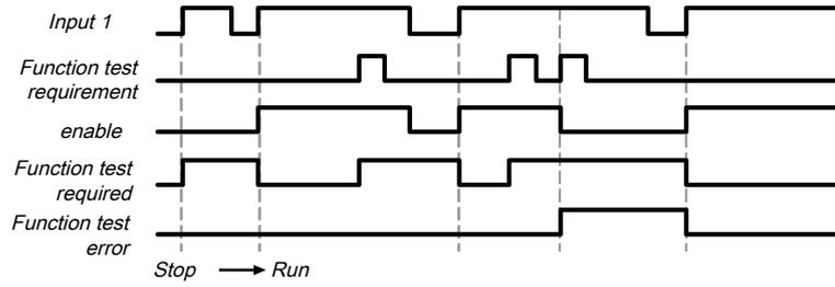
Illustration 110: Sequence/timing diagram for switch evaluation function block, category 2, single-channel with function test
