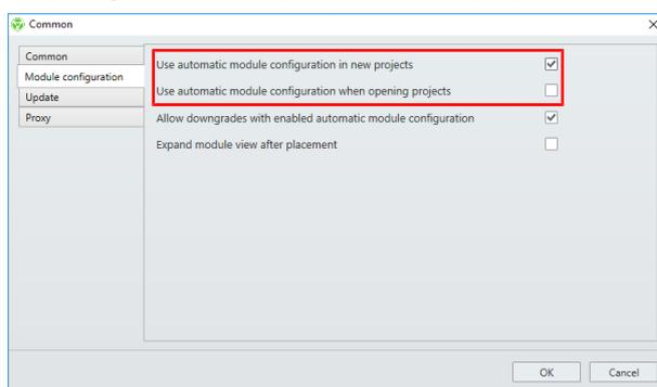
In this case, samos®PLAN6 always activates automatic module configuration for new projects. When you open an existing project, samos®PLAN6 automatically switches to manual module configuration.
