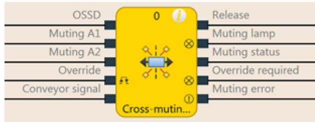
Illustration 129: Logical connections for the range function block Cross muting (two sides)
