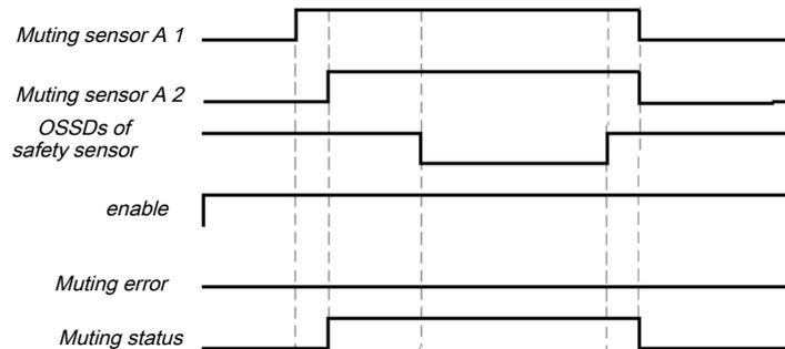
Illustration 128: Valid muting sequence when using the basic configuration setting
