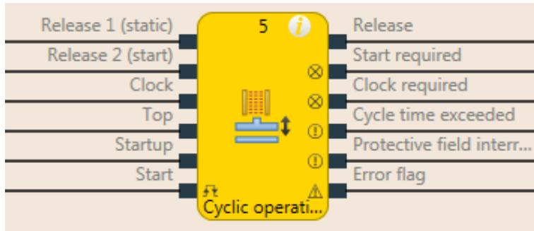
Illustration 157: Logical connections for the cyclic operation function block
