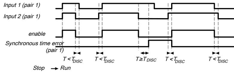
Illustration 111: Sequence/timing diagram for switch evaluation function block, category 4, two-channel without function test
