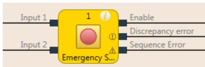
Illustration 105: Function block diagram for the emergency stop function block
