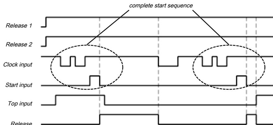
Illustration 163: Sequence/timing diagram if the Cycle input is low, startup muting inactive, and restart interlock set to 2 - always.
