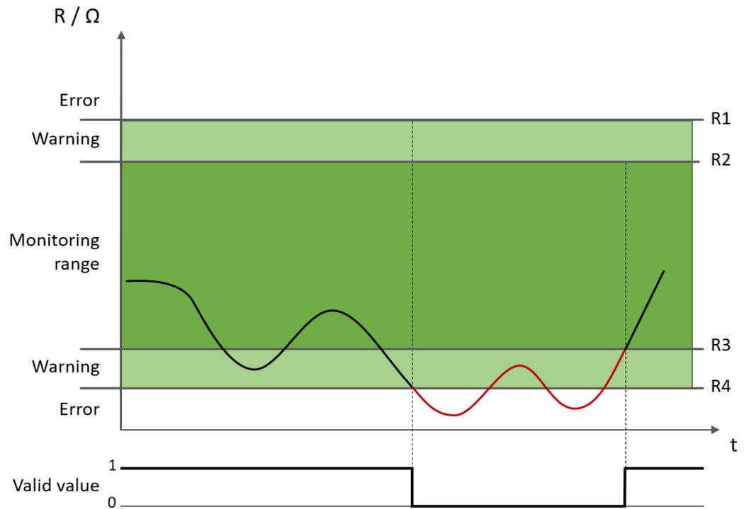
Illustration 42: Example: Value below lower limit of monitoring range (sensor RTD)
