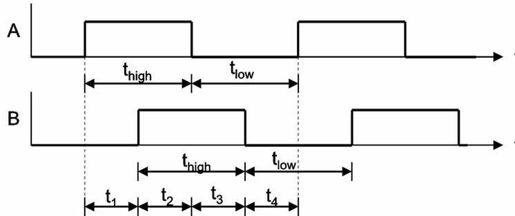
Illustration 99: Signal pattern for A/B pulse encoder with 90° phase offset
