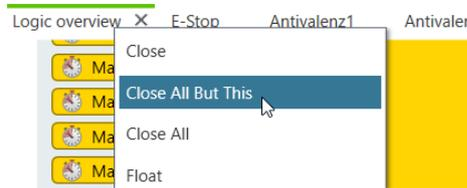
⇒ The **Logic overview** tab is the only tab that remains open in the working area.
