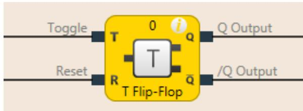
Illustration 52: Function block diagram for the T flip-flop function block
