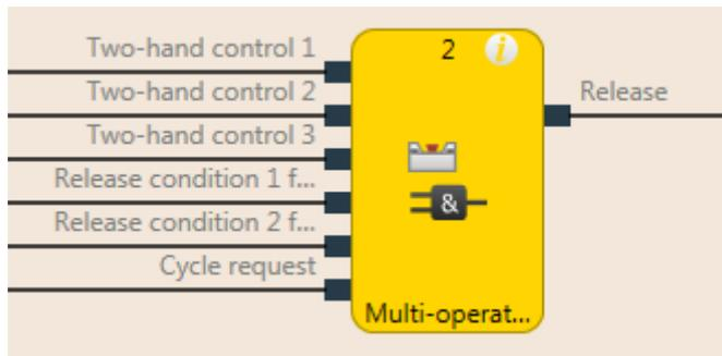
Illustration 115: Logical connections for the multi-two-hand function block
