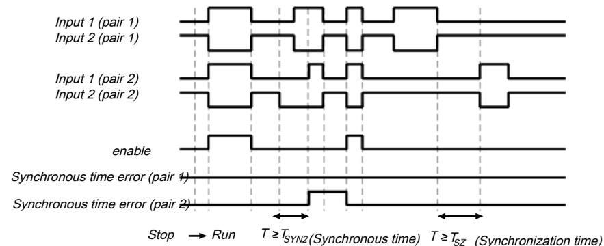
Illustration 114: Sequence/timing diagram for the two-hand type IIC function block
