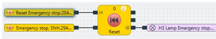
**Step 3: Parameterizing the logic module**
