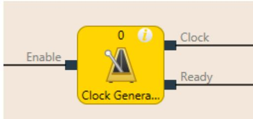
Illustration 55: Logical connections for the cycle generator function block
