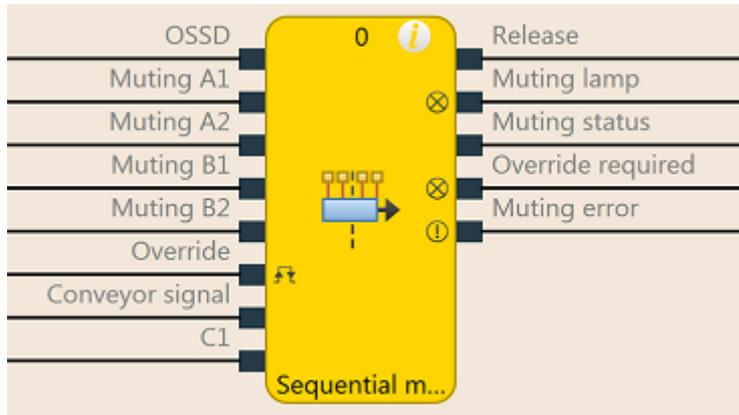
Illustration 123: Logical connections for the range function block Sequential muting
