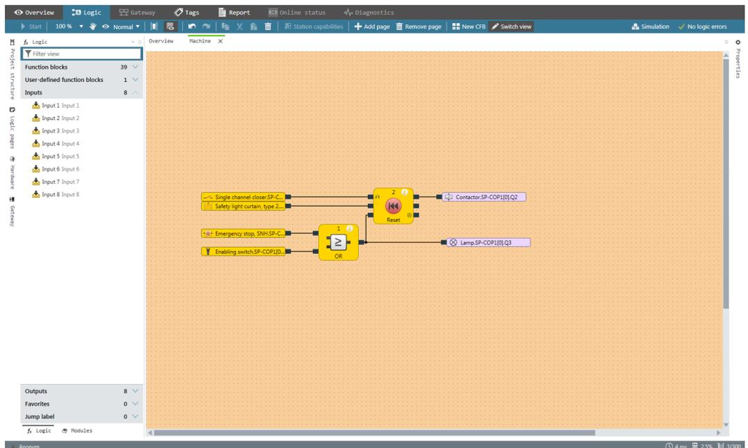
Illustration 32: Grouped function block with connected devices
