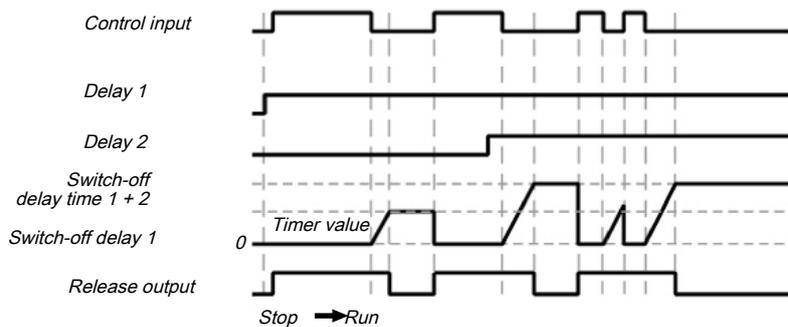
Illustration 85: Sequence/timing diagram for the adjustable switch-off delay function block with switch-off delay time 1 and switch-off delay time 2
