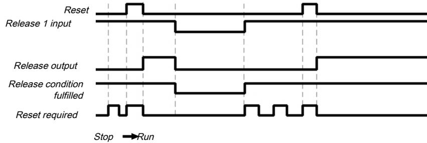
Illustration 79: Sequence/timing diagram for the reset function block
