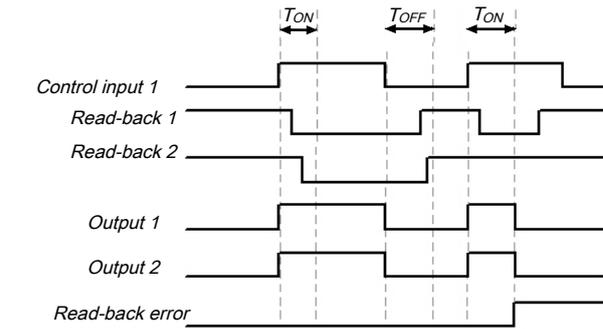
Illustration 94: Sequence/timing diagram for double valve in manual reset mode
