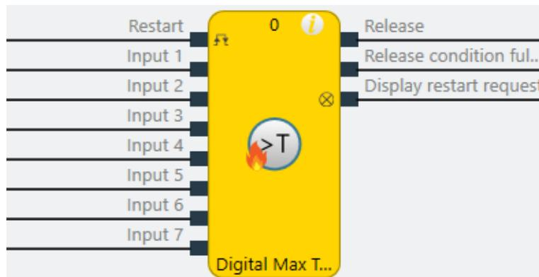
Illustration 214: Logical connections for the Digital max temperature function block
