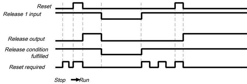
Illustration 215: Flow/Timing diagram for the function block
