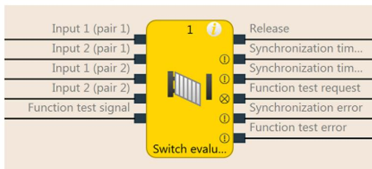
Illustration 109: Function block diagram for the switch evaluation function block
