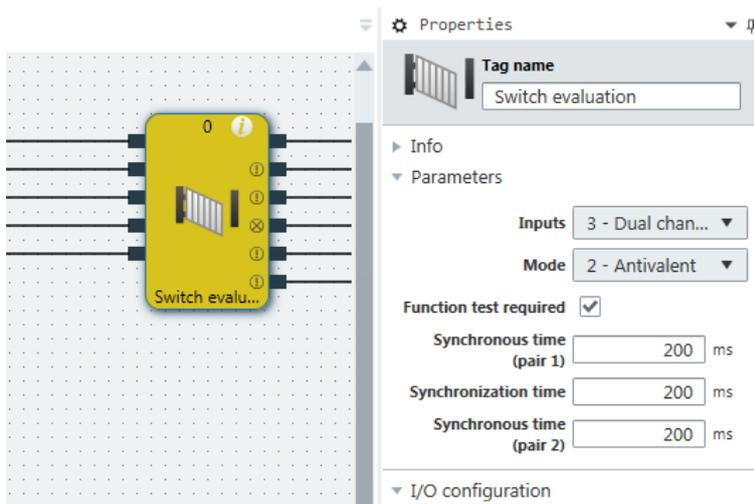
Illustration 45: Configurable parameters of function blocks
