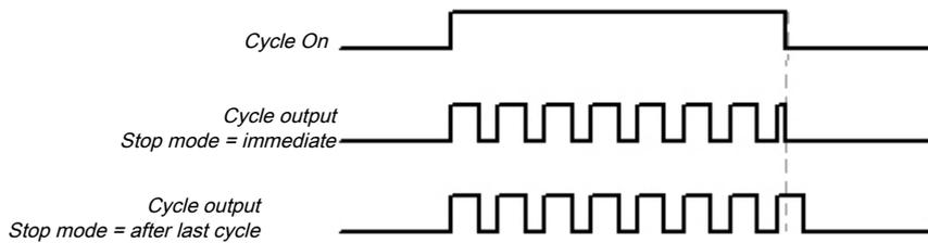
Illustration 57: Timing diagram for the cycle generator function block
