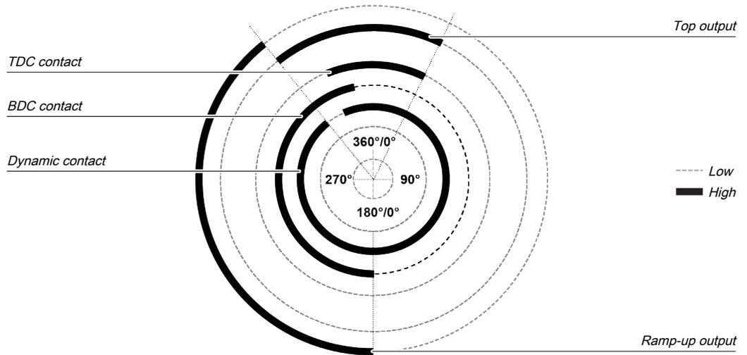
*Illustration 135: Press cycle for the eccentric press contact monitor function block with dynamic contact on the upstroke*
