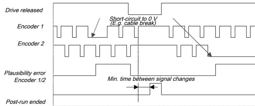
Illustration 104: Sequence/timing diagram for the ramp down detection with plausibility check function block
