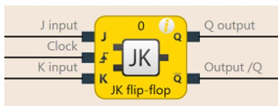
Illustration 54: Logical connections for the JK flip-flop function block
