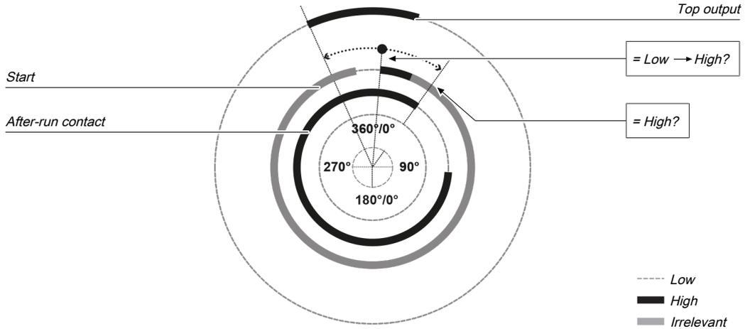
Illustration 144: Ramp-down monitoring with the universal press contact monitor function block
