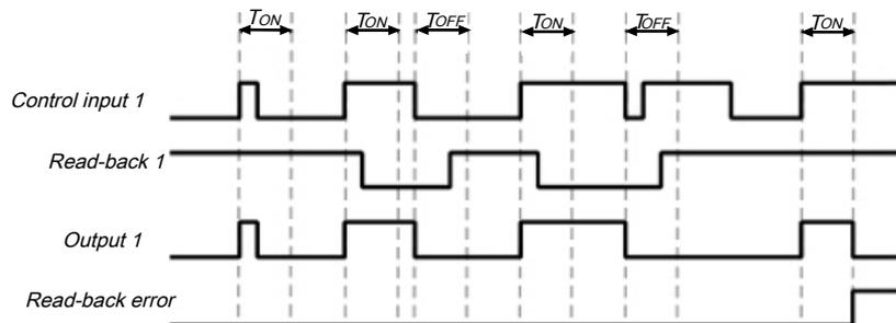
Illustration 93: Sequence/timing diagram for single valve in manual reset mode
