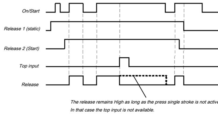
Illustration 149: Sequence/timing diagram for the press setup function block
