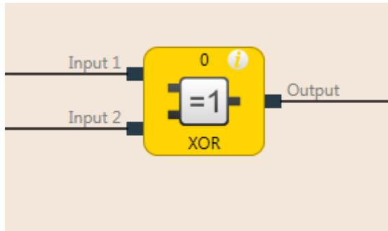
Illustration 51: Function block diagram for the XOR function block (exclusive OR)
