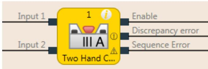
Illustration 112: Function block diagram for two-hand type IIIA function block
