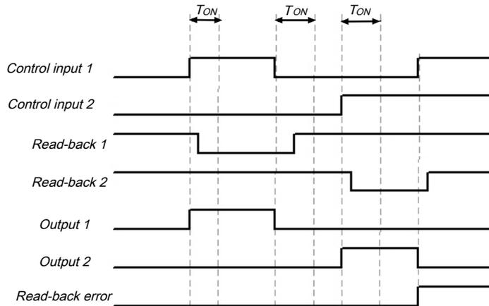
Illustration 95: Sequence/timing diagram for directional valve
