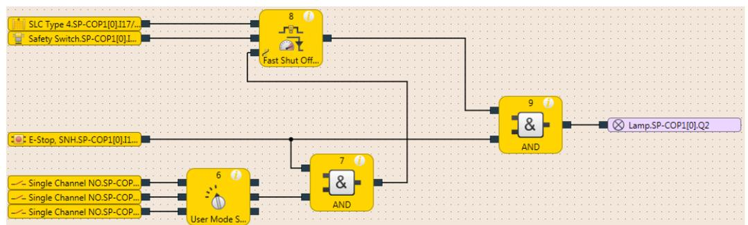
Illustration 66: Example of a fast shut-off with bypass with more than one condition for bypass
