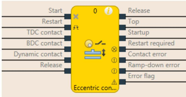
Illustration 132: Logical connections for the eccentric press contact monitor function block
