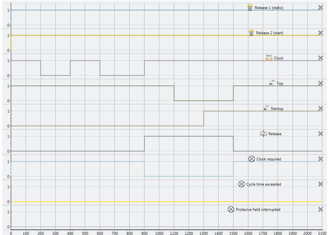
Illustration 158: Sequence/timing diagram for a complete sequence in standard mode with 2 programmed interventions without restart interlock.
