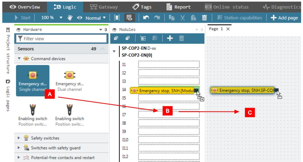
As you can see, for example: After just one operation, the selected sensor lies under **Modules** on the input of your choice and is ready for configuration at the same time in the **Logic** view.
