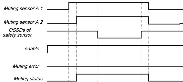
*Illustration 131: Valid muting sequence when using the basic configuration setting*
