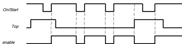
Illustration 153: Sequence/timing diagram for the press single stroke function block with configuration of On/Start to 1 - inching
