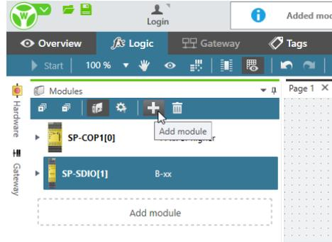
Manual interventions are usually only required if, for example, you want to add a second gateway module or extension module, although the previous configuration already has sufficient inputs and outputs.
