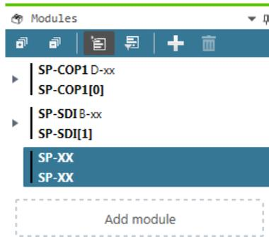
⇒ If required you can define additional options for the extended module in the **Properties** docking window.
