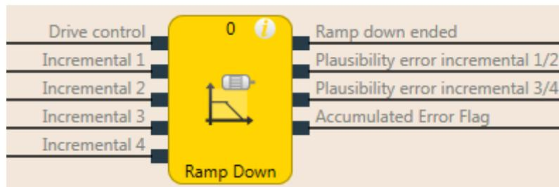
Illustration 98: Logical connections for the ramp down detection function block
