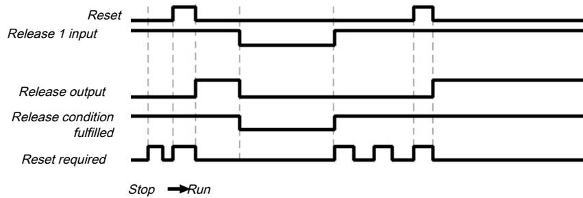
Illustration 219: Flow/Timing diagram for the function block
