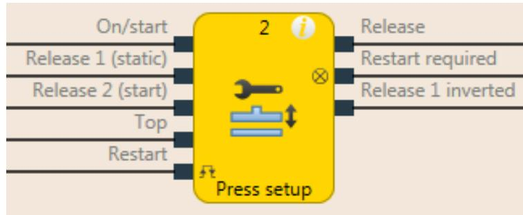
Illustration 147: Logical connections for the press setup function block
