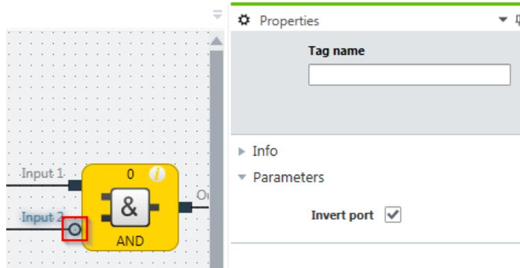
Illustration 46: An example of an AND function block with an inverted input
