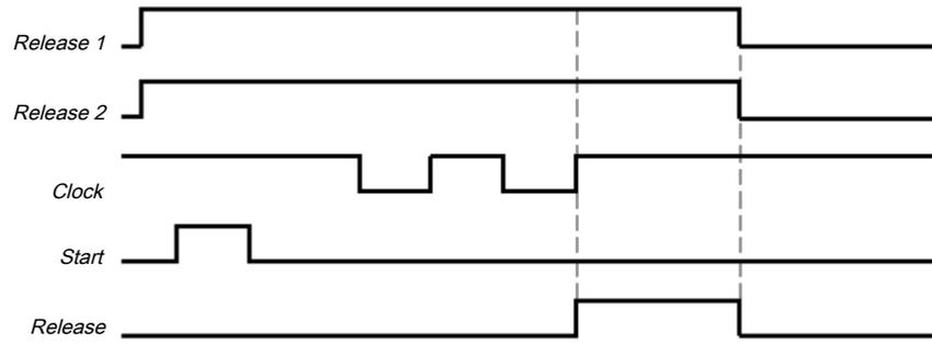
Illustration 160: Sequence/timing diagram for a complete start sequence in Sweden mode in two-cycle operation
