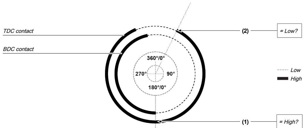
Illustration 140: Contact monitoring with the universal press contact monitor function block with activated BDC contact
