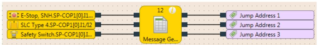
Illustration 73: Configuration example of a log generator with two emergency stop buttons and one safety switch
