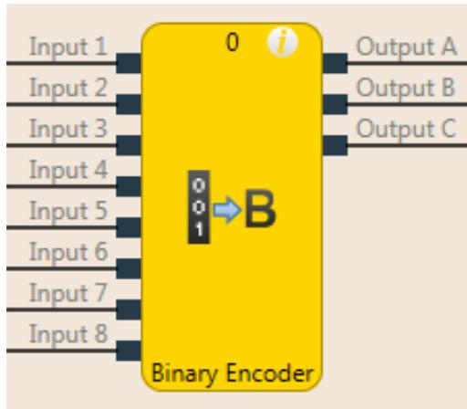
Illustration 69: Logical connections for the binary encoder function block
