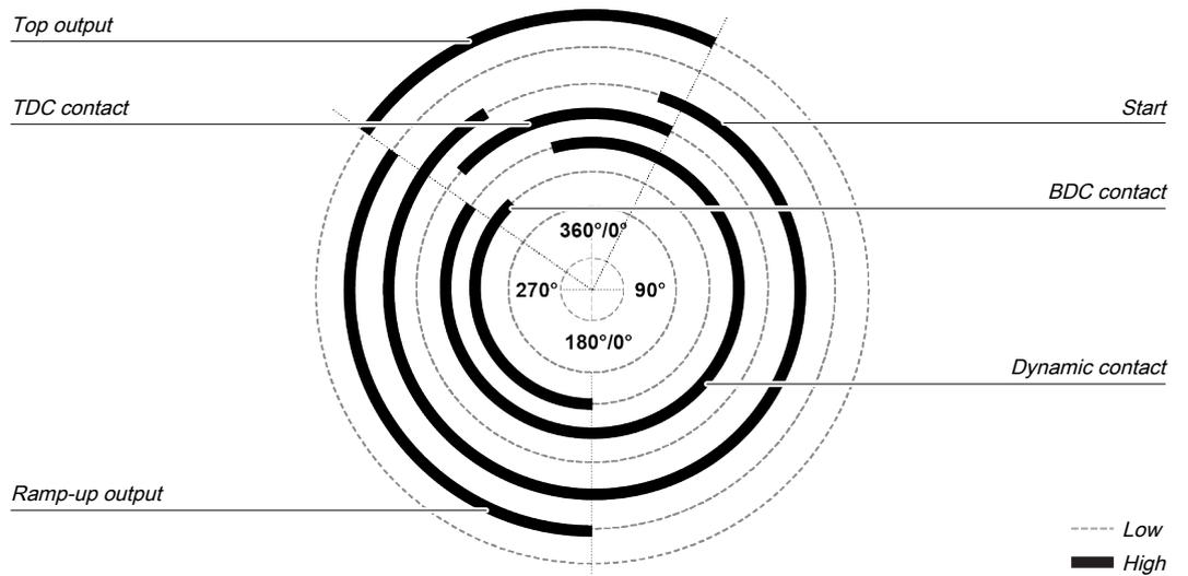
Illustration 137: Contact and output sequence of an eccentric press during an error-free sequence (example)
