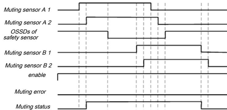
*Illustration 125: Valid muting sequence when using the basic configuration setting*
