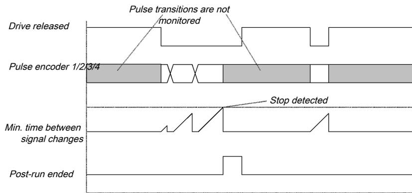
Illustration 103: Sequence/timing diagram for the ramp down detection function block
