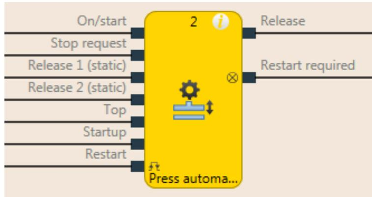
Illustration 155: Logical connections for the press automatic function block
