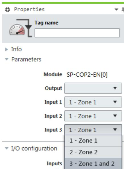
Illustration 63: Parameter settings for the fast shut-off function block
