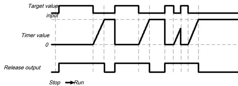
Illustration 83: Sequence/timing diagram for the switch-off delay function block
