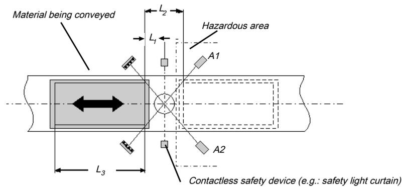
Illustration 130: Cross muting (two sides) with bidirectional movement of material
