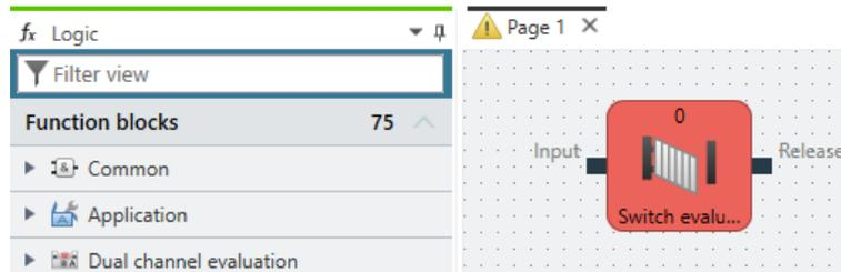
samos® PLAN6 automatically selects the minimum appropriate controller module for this control function. In this case, a controller module SP-COP1 in the required build state.
