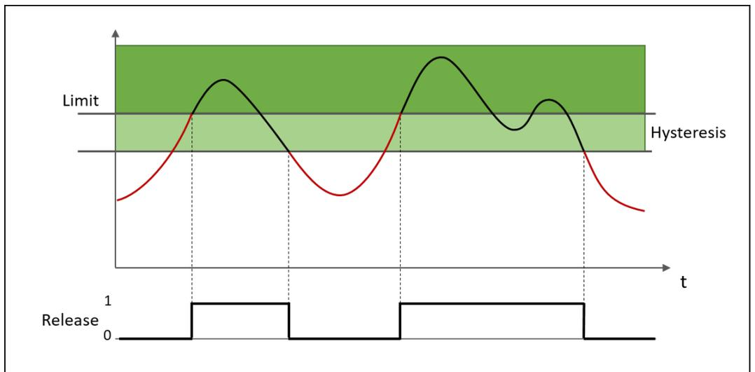
Illustration 183: Monitoring for "Lower limit exceeded"
