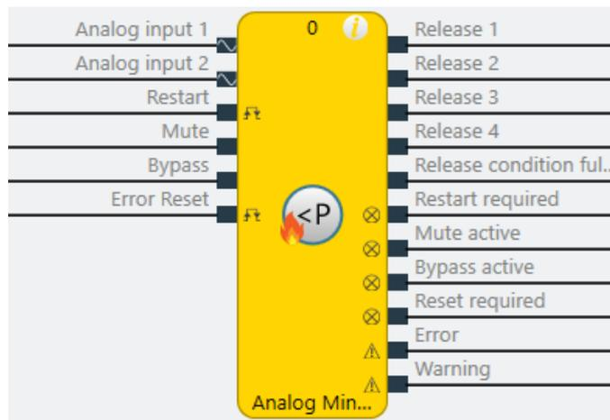
Illustration 181: Logical connections for Analog min pressure function block
