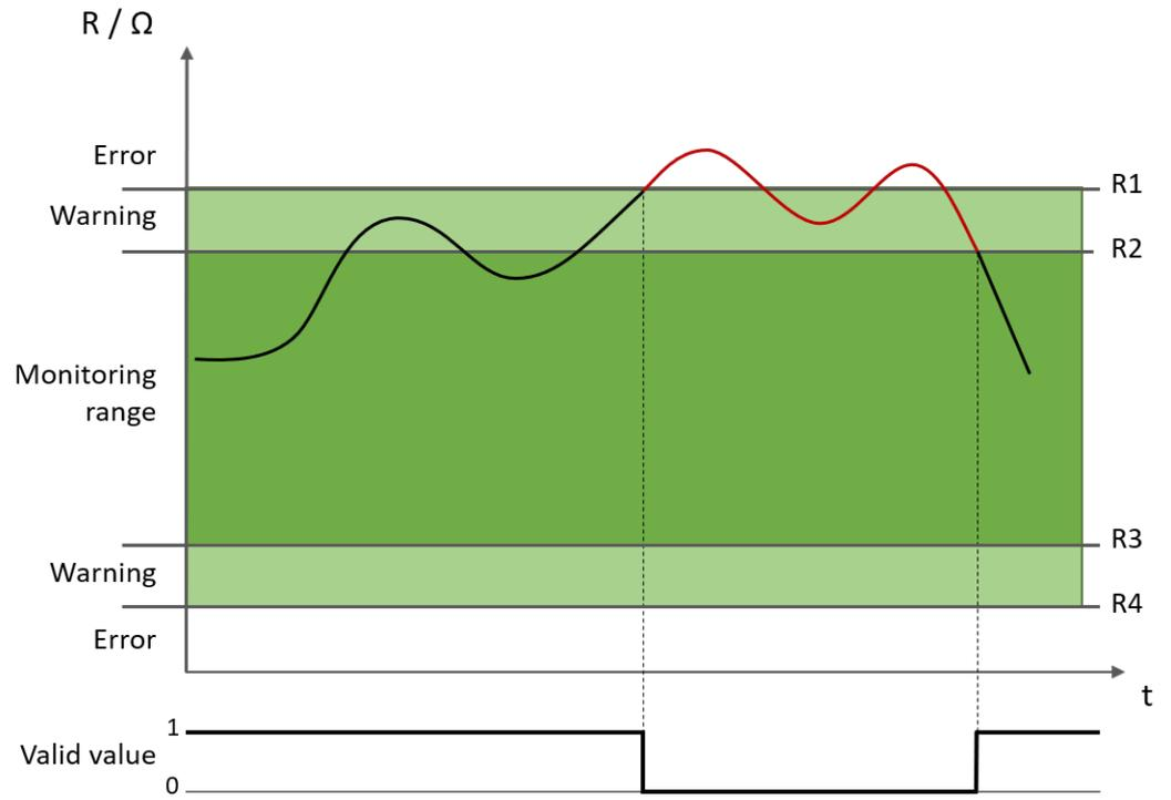
Illustration 43: Example: Value above upper limit of monitoring range (sensor RTD)
