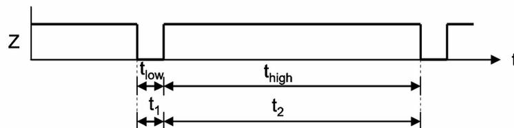
Illustration 101: Signal pattern for individual pulse encoder signal
