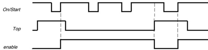
Illustration 154: Sequence/timing diagram for the press single stroke function block with configuration of On/Start to 2 - single start
