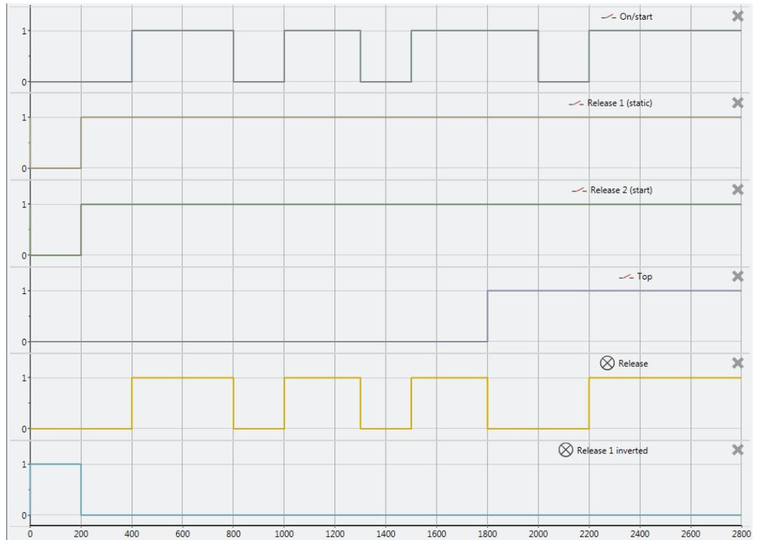
Illustration 148: Typical sequence/timing diagram for the press setup function block
