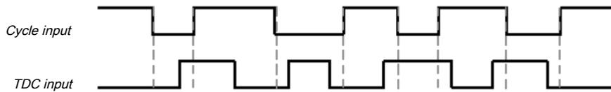
Illustration 162: Valid interventions if the Start of the first cycle parameter is set to 2 - After start of the startup.
