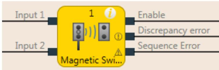
Illustration 107: Logical connections for the solenoid switch function block
