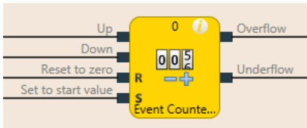
Illustration 58: Logical connections for the counter function block (up and down)
