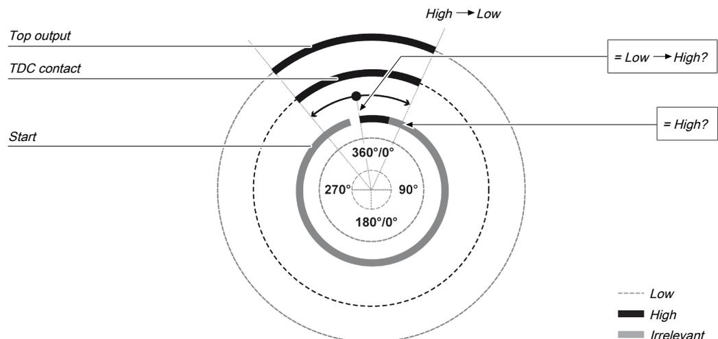
Illustration 134: Ramp-down monitoring with the eccentric press contact monitor function block
