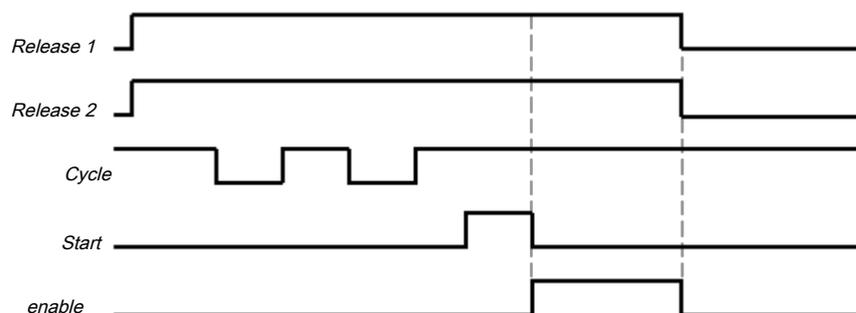
Illustration 159: Cycle/timing diagram for a complete start sequence in standard mode in two-cycle operation
