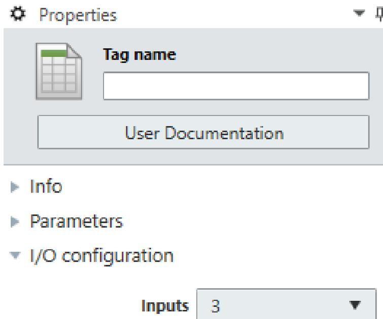
Illustration 74: I/O configuration for the log generator function block
