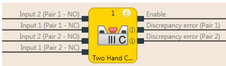
Illustration 113: Function block diagram for two-hand type IIIC function block
