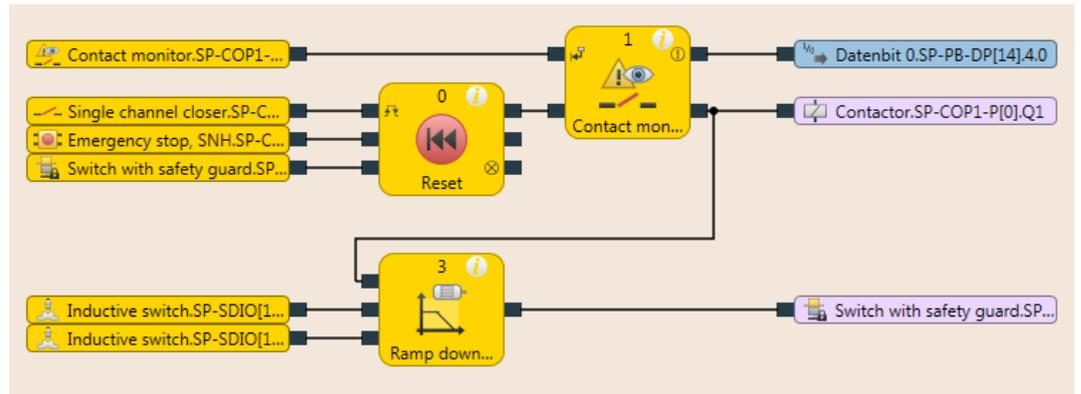
Illustration 102: Logic example of the "ramp down detection" function block
