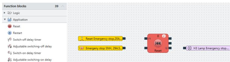
**Step 2: Connecting the inputs and outputs using the function block**
