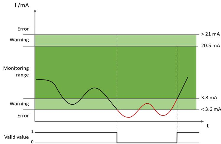
Illustration 40: Example: Value below lower limit of monitoring range (sensor 4-20mA)
