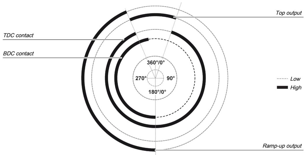
Illustration 141: Press cycle for the universal press contact monitor function block with falling edge of TDC contact before BDC contact
