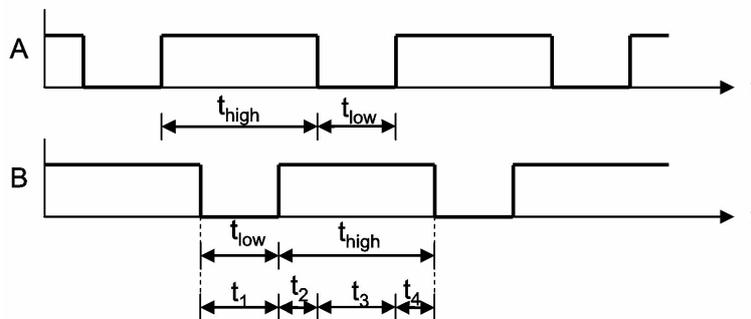
Illustration 100: Signal pattern for 1/3 gap pulse encoder with 180° phase offset
