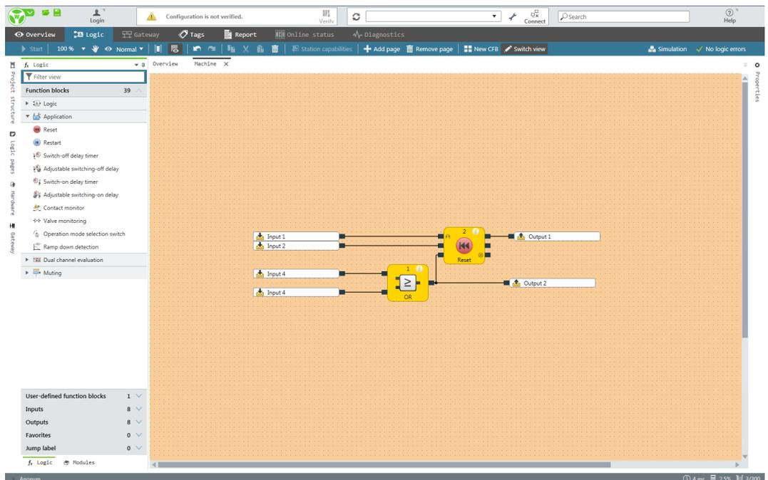
**This is how you can add inputs and outputs to a grouped function block.**
