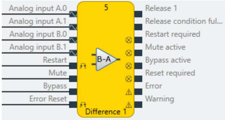
Illustration 175: Logical connections for the difference function block
