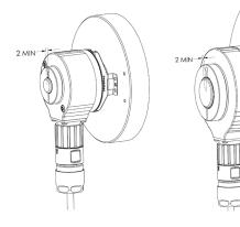
For safe clamping verify the driving shaft extends at least 2 mm out of the encoder. Check the position of the stator coupling. Avoid compressing or extending it to insure a minimal load on the bearing block.
