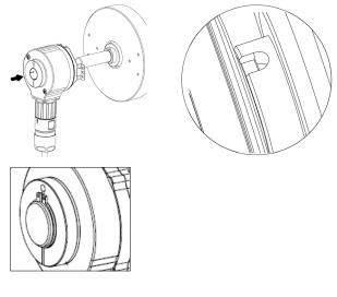
Check that the positive locks are in the correct position for proper engagement.
